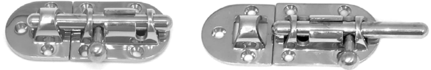
44.5455 Transom bolt / barrel bolt 4 3/8 inch; 316 stainless steel Overall: 110 X 38 X 19 mm; 4 3/8" x 1 1/2" x 3/4"; Throw: 1"
