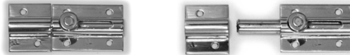
#92.080; small barrel bolt with strike plate; plate size: 50 x 36 mm 2" x 1 7/16"; strike: 30 x 36 mm; 1 3/16" x 1 7/16"; throw: 1 1/4". 304 stainless steel
